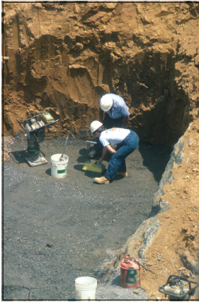
Compaction testing with radioisotopes
